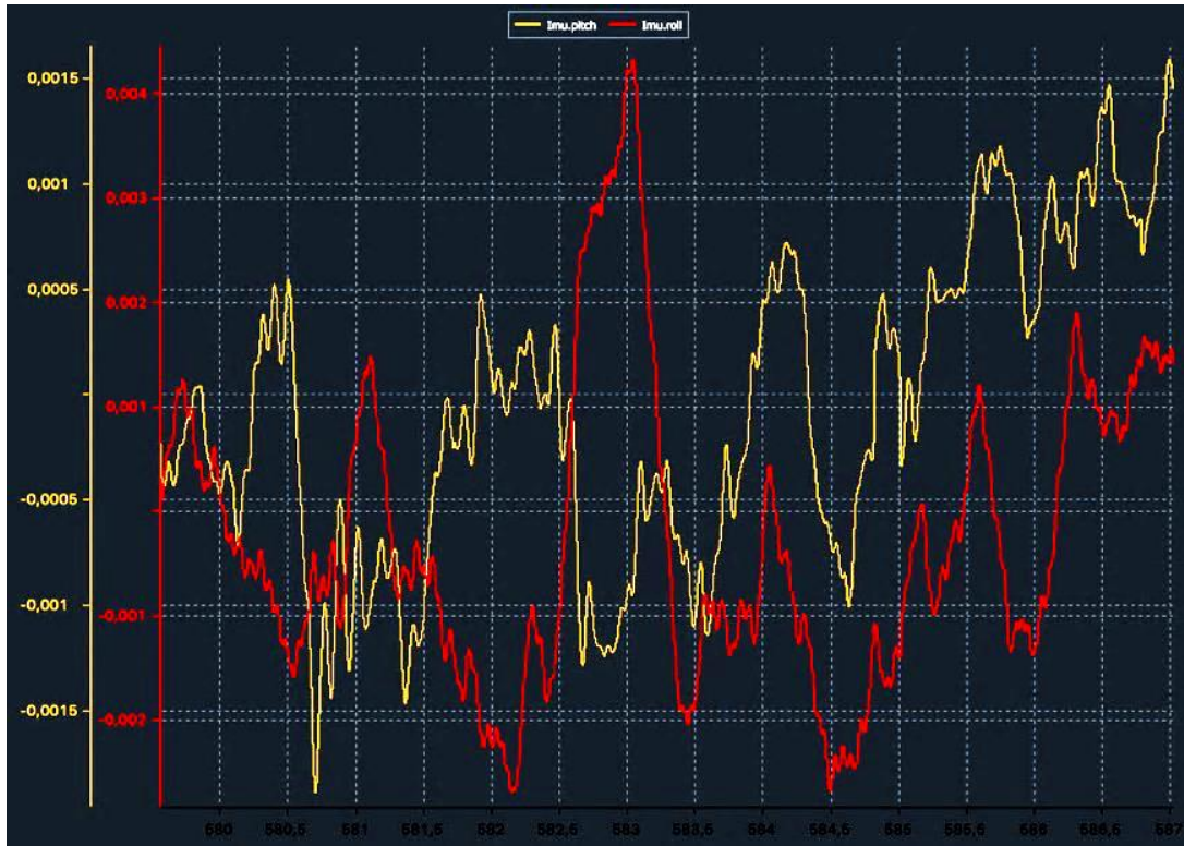
Figure 4.13: Steady-state noise on IMU roll (red) and pitch (yellow). Vertical: IMU values in radians. Horizontal: Elapsed time [0.5s/div].
