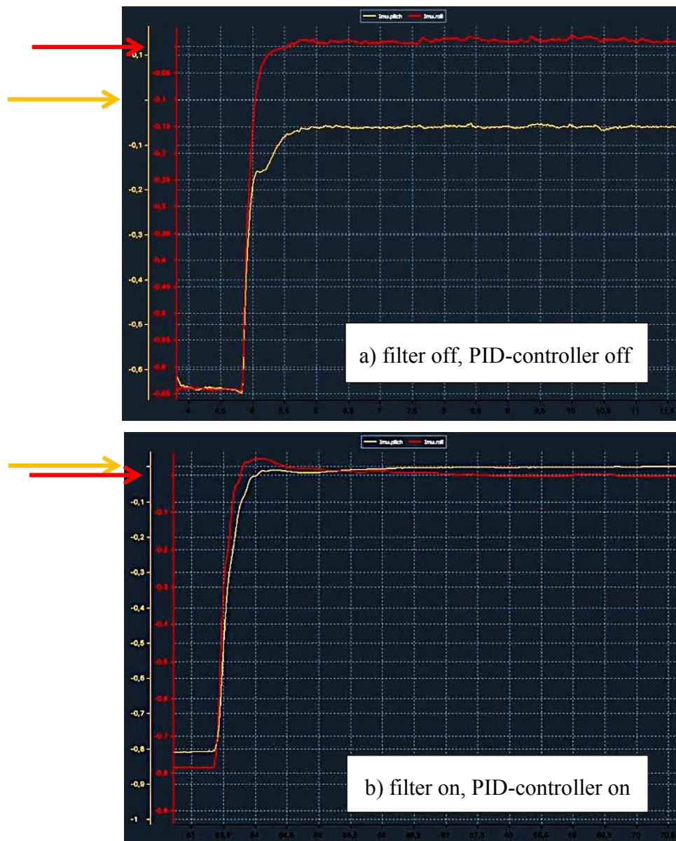
Figure 4.12: Graphs showing the effects turning digital LPFs and PID-controllers on/off. The red and yellow lines represent the measured roll and pitch respectively, while the red and yellow arrows indicate the setpoints for these signals. Vertical: IMU values in radians. Horizontal: Elapsed time [0.5s/div].
